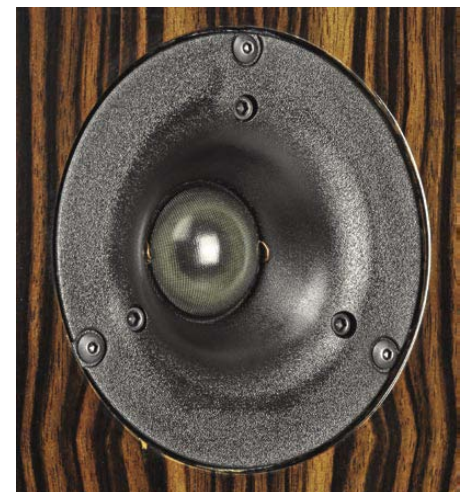
The 1in (25mm) silk dome tweeter sits in a shallow horn to improve sensitivity.
